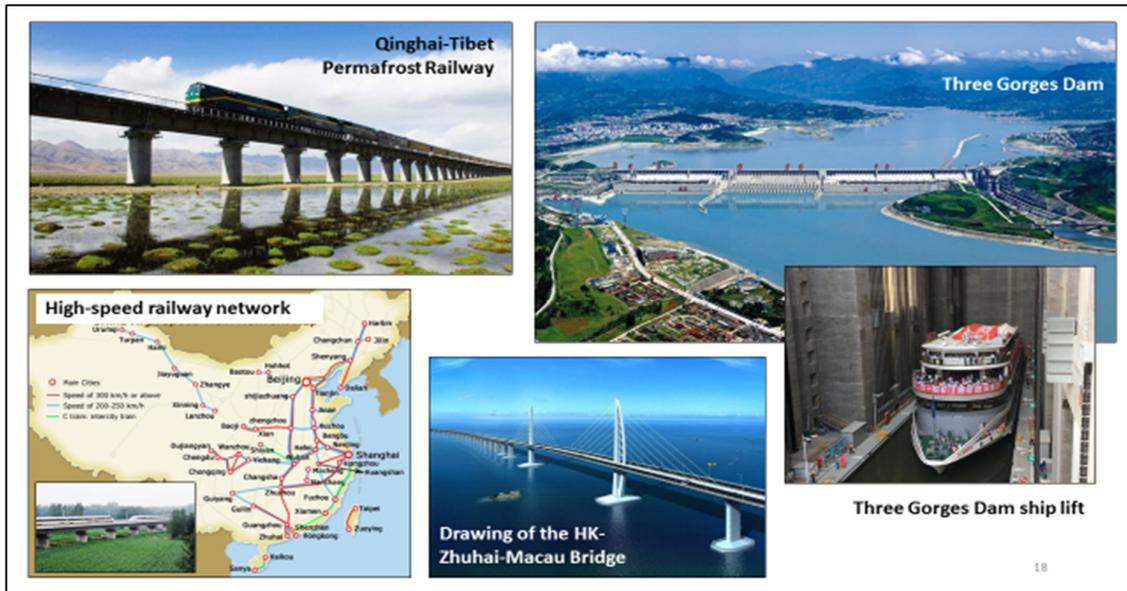
46. Take Permafrost railway for example: it presents multiple engineering challenges. Permafrost melts with slight changes in temperature – heat from trains can also cause melting. Permafrost thaws, ground becomes muddy, affecting integrity of entire system. For fragile sections, Chinese engineers built elevated tracks with pile-driven foundations sunk deep into the ground. And China has built an impressive rail network on Permafrost – quickly as well.
