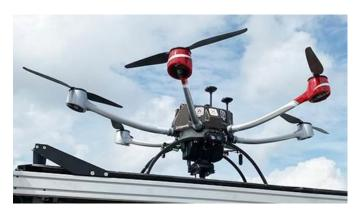
HTX's newest unmanned aerial vehicle is capable of long-distance flights without the need for a safety pilot, offering officers a real-time situational picture of incident sites and a bird's-eye view from kilometres away.
