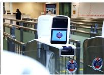
Since July, our land, sea and air immigration checkpoints have been equipped with iris and facial scanners, providing a more secure and efficient means of traveller identity authentication. The **Multi-Modal Biometric System (MMBS)**, which enables the use of iris, facial and fingerprint biometrics for immigration clearance, was developed to centralise all biometric services and data to support ICA's biometric needs.
