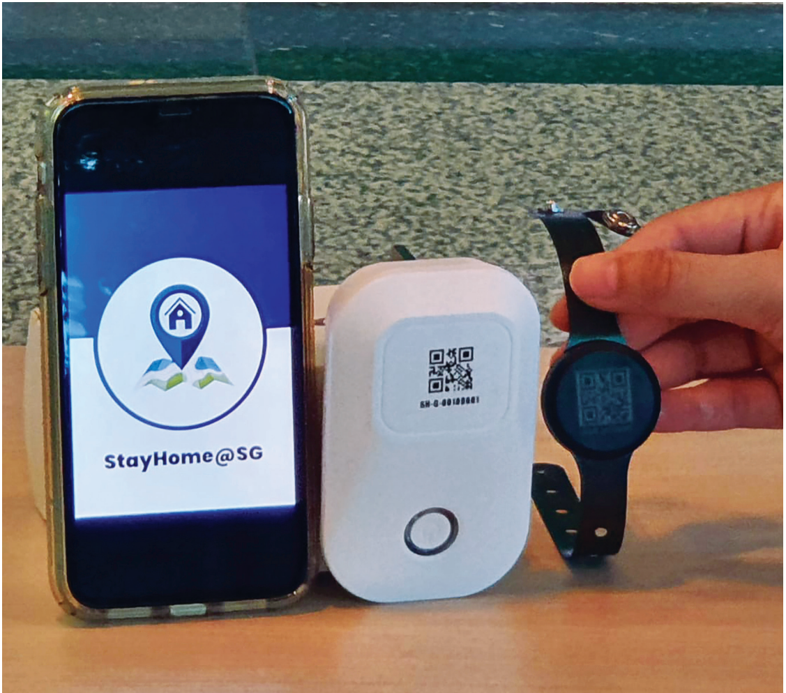
Figure 4. (Left to right) mobile application, IoT gateway and wristband deployed for SHN electronic monitoring
