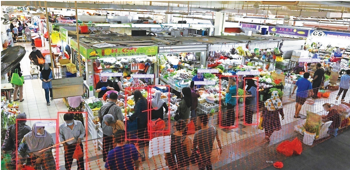
Figure 3. Crowd analytics algorithm tested on a semi-crowded scene. Safe distancing violations are annotated by the red bounding boxes.
