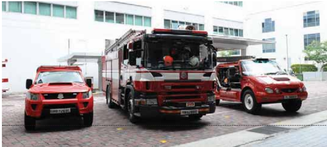
The concept of a fire-fighting vehicle – (left) latest Red Rhino developed in 2009 (middle) traditional fire engine or Pumper (right) first generation of Red Rhino developed since 2000
